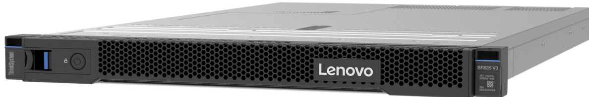
Figure 20. Lockable front security bezel
